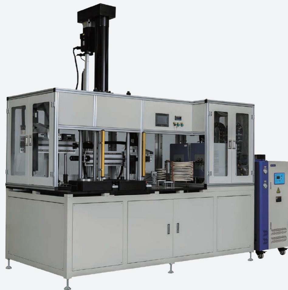
Automatic Shrink Fitting System for stator and rotor
