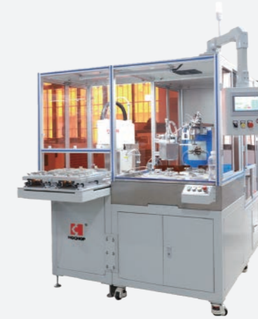
Induction Brazing Machine for Electrodes Brazing of Car Battery
